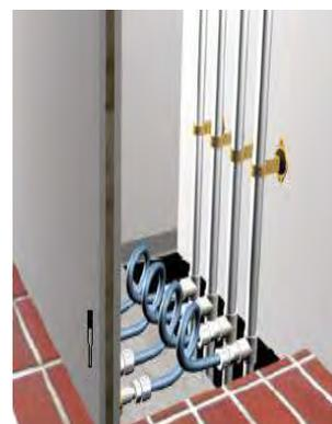
Fig 4. Conectores flexibles
